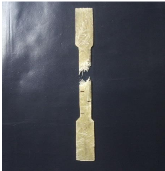
Figure.2. Failure of specimen after tensile
