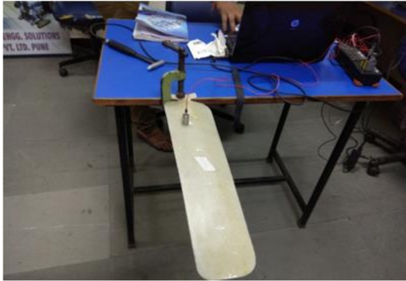
Figure.10. Clamping Fibre glass Blade using C-clamp
