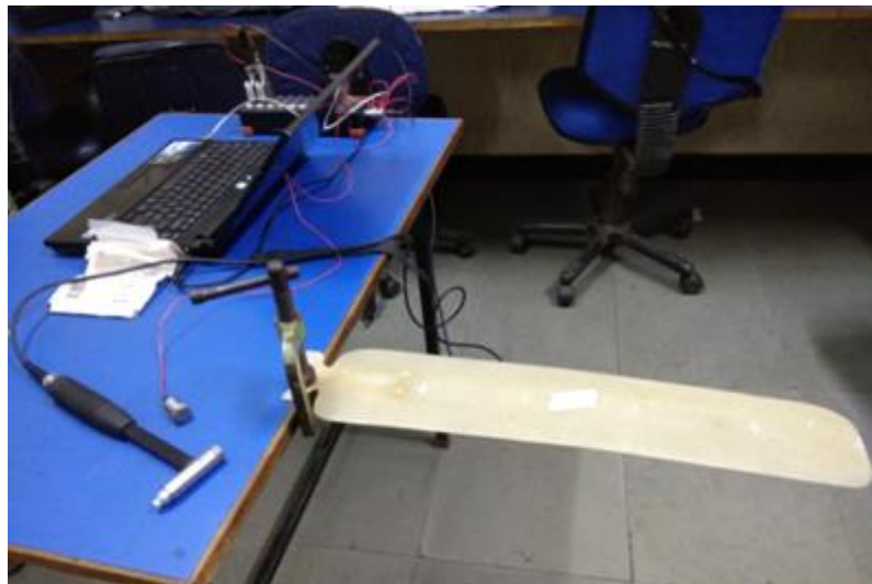
Figure.9. Clamping Fibre glass Blade using C-clamp
