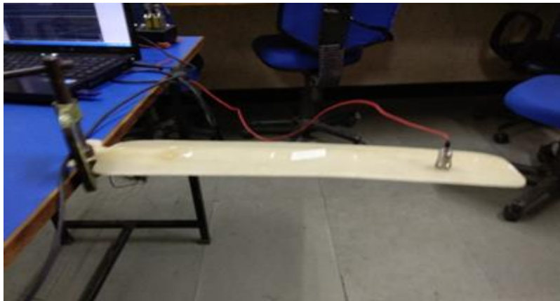
Figure.11. Accelerometer is attached to fan blade for measuring natural frequency at last mode point
