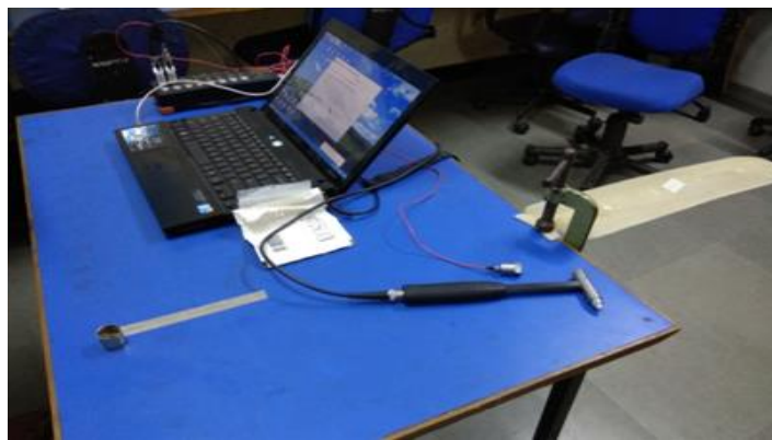
Figure.8. Vibration testing Experimental Setup
