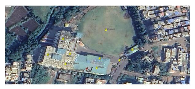
Nine points were selected based on best suitable requirement for noise monitoring. RS-2250 instrument was used. Monitoring was carried out 3 times in a day for 3 months. Readings were collected in morning section, afternoon section and evening section. In addition to this monitoring was also carried out in library section, study room section, classrooms, tutorial rooms and laboratories.
