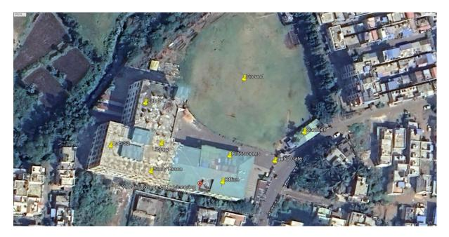
Nine points were selected based on best suitable requirement for noise monitoring. RS-2250 instrument was used. Monitoring was carried out 3 times in a day for 3 months. Readings were collected in morning section, afternoon section and evening section. In addition to this monitoring was also carried out in library section, study room section, classrooms, tutorial rooms and laboratories.
